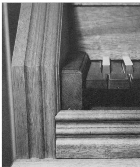
The horizontal moulding under the keyboard attached to the cheek did not please me because of the pretty profiles not fitting correctly there according to the construction manual (left photo). I therefore found a different solution (right photo), which, however, required to have an additional piece of the moulder rail sent to me.
