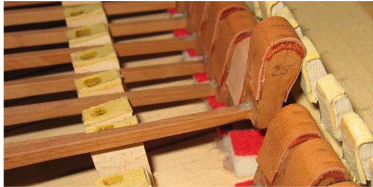
One recognizes above how the catching piece holds the hammer head. The photo at the left shows the individually adjustable backcheck (left, in its normal position) and on the right of it for comparison the continuous backcheck.
